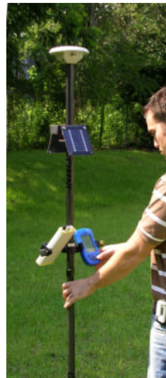
Figure 3. DataGrid Mk-1 Crane or Toughman GPS/Data collectors in typical field configuration. Shown on a pole with low weight antenna, solar panels and a PDA.
